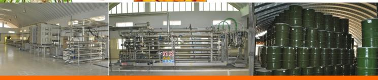
HACCP: The Processing units of TMN International are well equipped with state of the art machinery with washer, destoner, pulper, decanter, seperator, evaporater and filling machines for Aseptic and OTS cans. The process is carried out in temperature controlled sheds- fruits are examined on converyer system and after pulp, the process is carried out through SS pipes, product sterlised, cooled and filled based on the principles of Hazard Analysis and Critical Control Point (HACCP).
